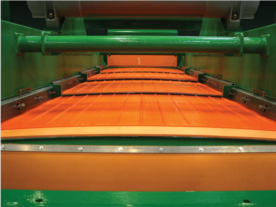
The fine polyurethane shale shaker screen mesh with trapezoidal hole could resist small particles blinding.
