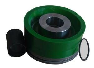
The Green Duo piston is a bonded dual durometer piston that is highly resistant to abrasion and tear. The bonded construction resists extrusion under pressure and restricts movement to reduce the build-up of heat.
